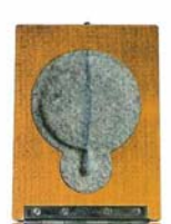
Seikosa artillery chronographs: Figures 54 to 56, left to right. The marking on the back of this artillery chronograph translates as "Air Corps second watch type 1."
