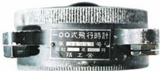
Figures 35 to 38, clockwise from top. Seikoshia aircraft clock with central seconds, turnable bezel, and two colored elapsed time indicator marks. The dial is signed with "TOKI" (time), the case is of light metal, and the tag markings translate as "type 100 aviation clock no. 2481."
