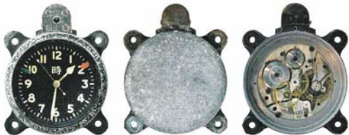
Figures 35 to 38, clockwise from top. Seikoshia aircraft clock with central seconds, turnable bezel, and two colored elapsed time indicator marks. The dial is signed with "TOKI" (time), the case is of light metal, and the tag markings translate as "type 100 aviation clock no. 2481."
