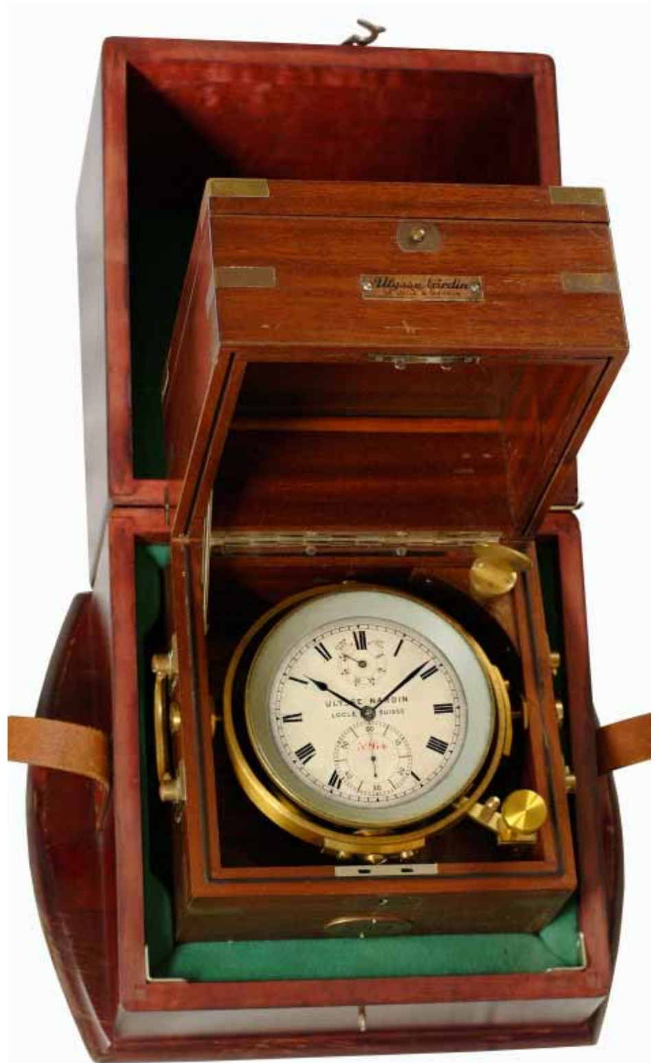
- Ulysse Nardin Ships chronometer No. 5264 of the WWII 'Kriegsmarine' with eagle and swastica and navy registration no. M 1848 gimballled in mahagoni case.
