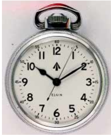
Elgin deck watch of the Royal Navy: chromed case, screwed back, second hand stop device, 21 jewels, adjusted in 5 positions and temperatur, Cal. 581 B.W.Raymond, no. 41752745, stock order no.: ^ Ser. No. 51389.
