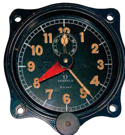
An aircraft instrument-panel clock; this one, an Omega, number 592721 is dated 9 August 1936. Made to specification FI.22601.
