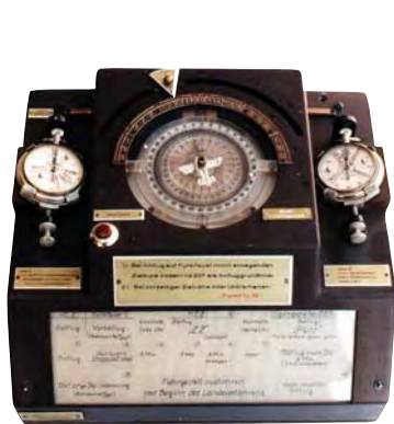
Above left: A target finding device with two Junghans special stop watches marked with the Luftwaffe test centre Redclin no 85065 and 850657. This device was used for training pilots.
