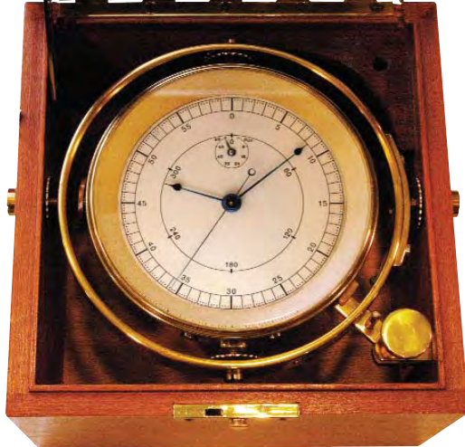
A Lange & Söhne no. 650; an early timing instrument for the German Airforce, four-pillar movement, with hour angle dial, and an external safety hand-setting device. Supplied as a surface chronometer for airfields.
