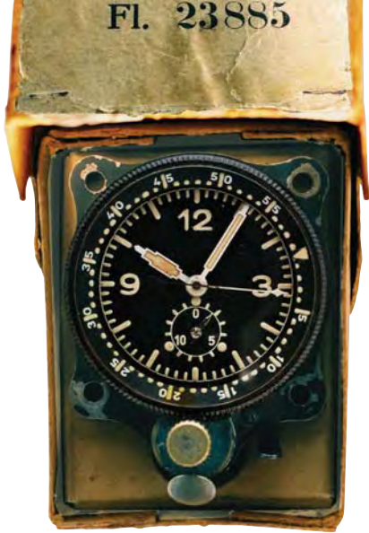
A Junghan blind-flight clock, with chronograph function and fifteen-minute recorder. The specification number is visible on the box lid.
