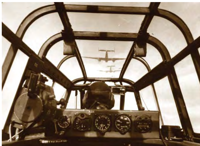
Cockpit of a Me 110. The instrument panel has, on the left, a Junghans Bo UK 1 spec FI. 23885, movement J30BZ with 15 min or 30 min counter.
