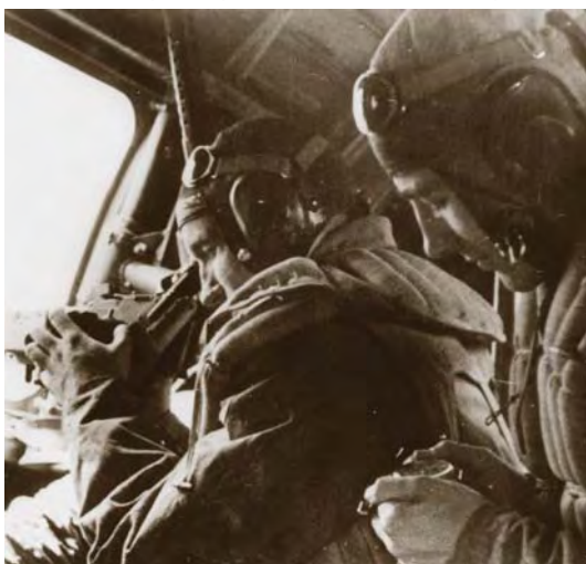
Astronomical positioning on a long-range flight using a bubble octant and an aerial navigation wristwatch.
