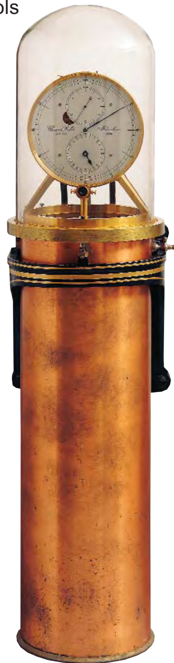
High Command. Regulators such as this one by Riefler, no. 368, defined the standard time, disseminated by the Observatory, and used for rating military chronometers.
