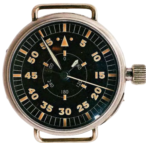
A later Lange & Söhne Luftwaffe hour angle watch, gilt three-quarter plate movement, base cal. 43, in a silver case, marked 92665. Luminous hands for degrees, minutes and radial four-degree indication.
