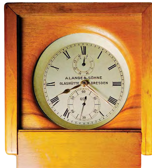
A Lange & Söhne Luftwaffe chronometer no. 659, supplied on 24 June 1936. Spring detent escapement, nutwood box with sliding top. There are no gimbals but the clock is pivoted along its 12-6 axis.
