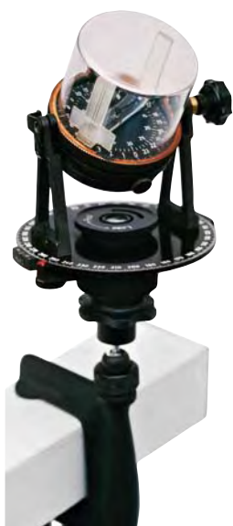
Above left: Sun compass C Plath Hamburg. There is an integrated 24h clock, Junghans cal J30 E, 8 days, device no 127-1676A1, no 510, producer code, 'gtl', on top of the clock.
